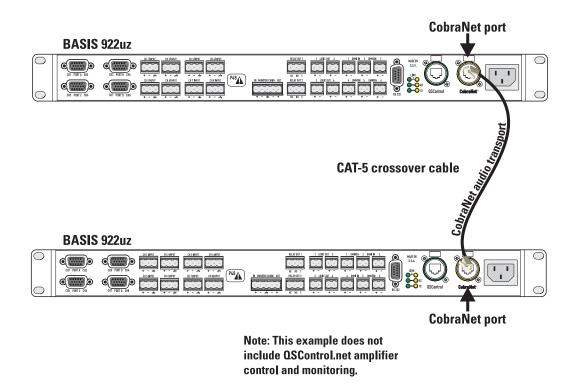
Combining example 1 and 2 lets you setup and monitor one box at a time, much as you would have to do using a point-to-point RS232 connection, while passing audio between them, all without a network switch. However, you would have to physically connect your computer first to one BASIS box and then to the other. With this elementary connection you don't have a true network. It is just like making RS-232 connections - except that performance is much better.
