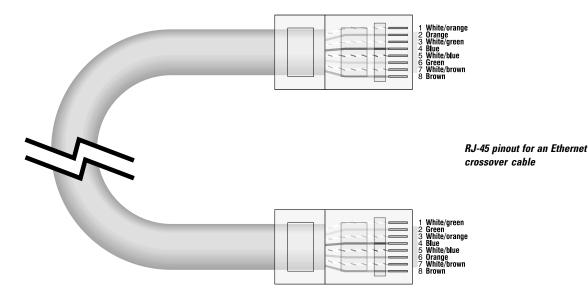
The wire in UTP cabling is twisted together in pairs. Rather than randomly choosing a wiring scheme for the networking cable, it is important to have the RX wires in one pair and the TX wires in another pair, especially in longer cable runs.
